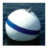
Mooring buoys are used to anchor/moor boats and/or floating docks. In compliance with national standards, mooring buoys shall be white, circular or cylindrical, and have a 2 inch, blue horizontal stripe.
